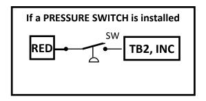
Be sure that the WT500 is programmed to monitor the PRESSURE SWITCH input terminals PS1-PS2. In the INITIAL SETUP procedure, set: 2ND STG = 1
